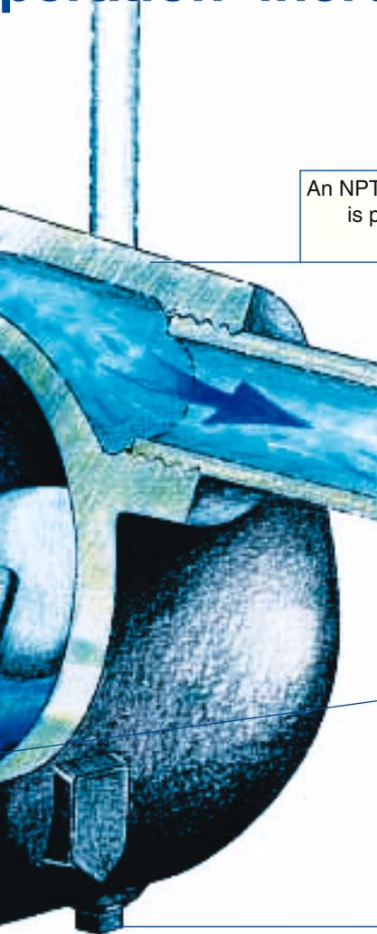
An NPT balance pipe tapping is provided in the top of the body
