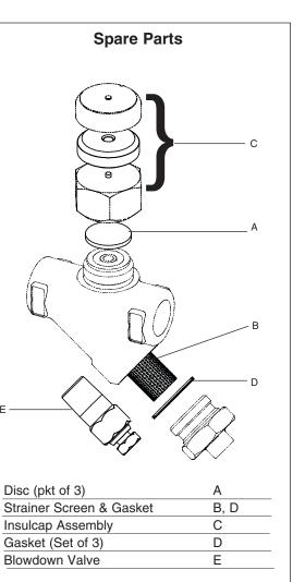
Available spare parts are shown in heavy line. Parts drawn in broken line are not supplied as spares.
