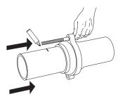
2. Assemble push-on joint using standard procedure. Insert one of the extra long T-Bolts (provided) through one of the bell ring holes. Mark a line on the pipe approximately 1 inch shorter than the bolt length.
