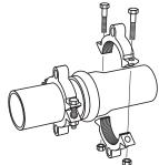
2. Assemble Series 1390 clamping rings onto spigot pipe and just 3. Insert all provided connecting rods and nuts as shown and behind bell end as shown (use restraining rods as a guide to position and align restrainers) and tighten bolts and nuts evenly to at least the minimum recommended torque (see table). A torque wrench is required to ensure proper torque.
