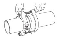
4. Insert all provided T-Bolts and connecting rods. Snug nuts behind restrainer ears as shown above. Do not over-tighten retaining nuts.
