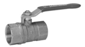
Threaded Series 351T and 356T are the most economic choice for general purpose ball valves from Jamesbury. Sizes range from 1/4" – 3" (DN 6 – 80). Series 356T features 316 stainless steel ball and stem which is ideal for saturated steam service to 150 psi (10.34 bar).
