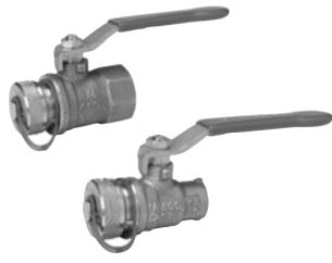
Series 361T and 362T valves feature a 3/4" male hose thread. The hose end includes a cap with lace retainer. Available in 1/2" and 3/4" (DN 15 and 20) sizes. Series 361T has female NPT, and 362T is made for joining with solder. Excellent valve for utility services such as water and HVAC. The hose connection is great for washdown and drain.
