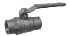
Solder End Series 341T and 346T are available in 1/2" - 2" (DN 15 – 50) sizes. Series 346T Features 316 stainless steel ball and stem.
