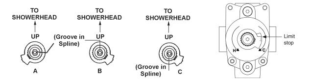
3. If the desired position falls between adjacent positions on the spline, flip the stop over so that the other face shows. This shifts the stop position by 1/2 spline.
