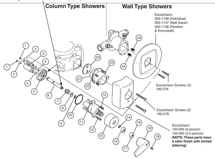
Valves are equipped with a temperature limit stop which can be used to limit the temperature of tempered water discharged. To adjust the temperature, remove the handle and loosen the set screw. remove the limit stop and reposition to desired setting. Turn the limit stop counterclockwise for a hotter setting and clockwise for a cooler setting.
