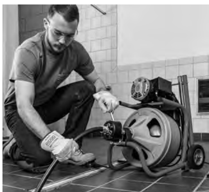
Figure 16 – Using Machine with Guide Hose
