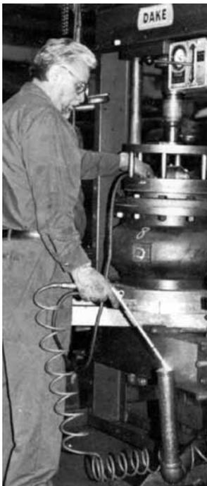
All APCO Silent Check Valves 100% hydrostatically tested to ANSI standards
