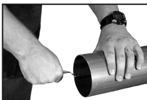
Figure 3: Deburr inside diameter deburring tool
