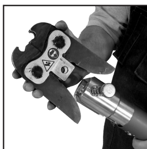
Figure 7: Placement of adapter jaw into the tool
