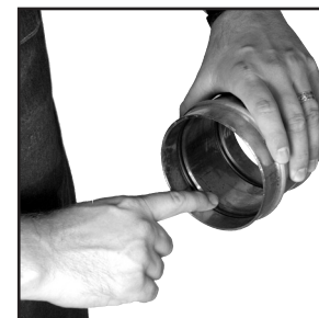
Figure 5: Check for EPDM seal
