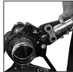
Figure 8: Placement of adapter jaw into pressing chain
