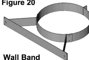
18. Fasten the wall band securely around the chimney with the supplied nut and bolt. Check for clearances and plumb as you fasten the wall bands to the wall. Use a level against the chimney sections at each support stage to keep the assembly plumb.
