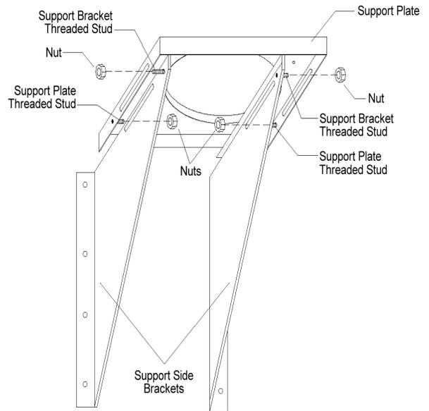
**Underside View of Threaded Studs and Nuts**
