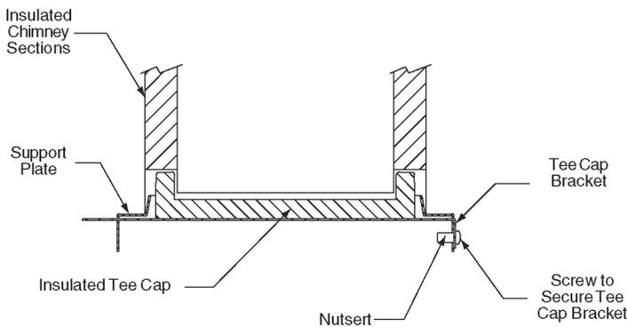
**Securing of Insulated Tee Cap**
