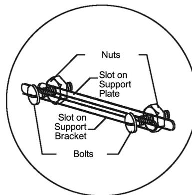
**Slot Areas with Bolts (#8 x 3/4") and Nuts Assembly of Support Brackets and Support Plate**
