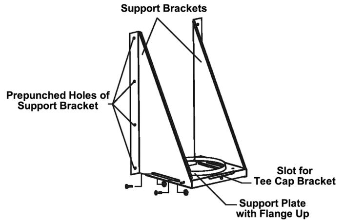
**Front View of Wall Support Assembly with Brackets Mounted above the Support Plate**
