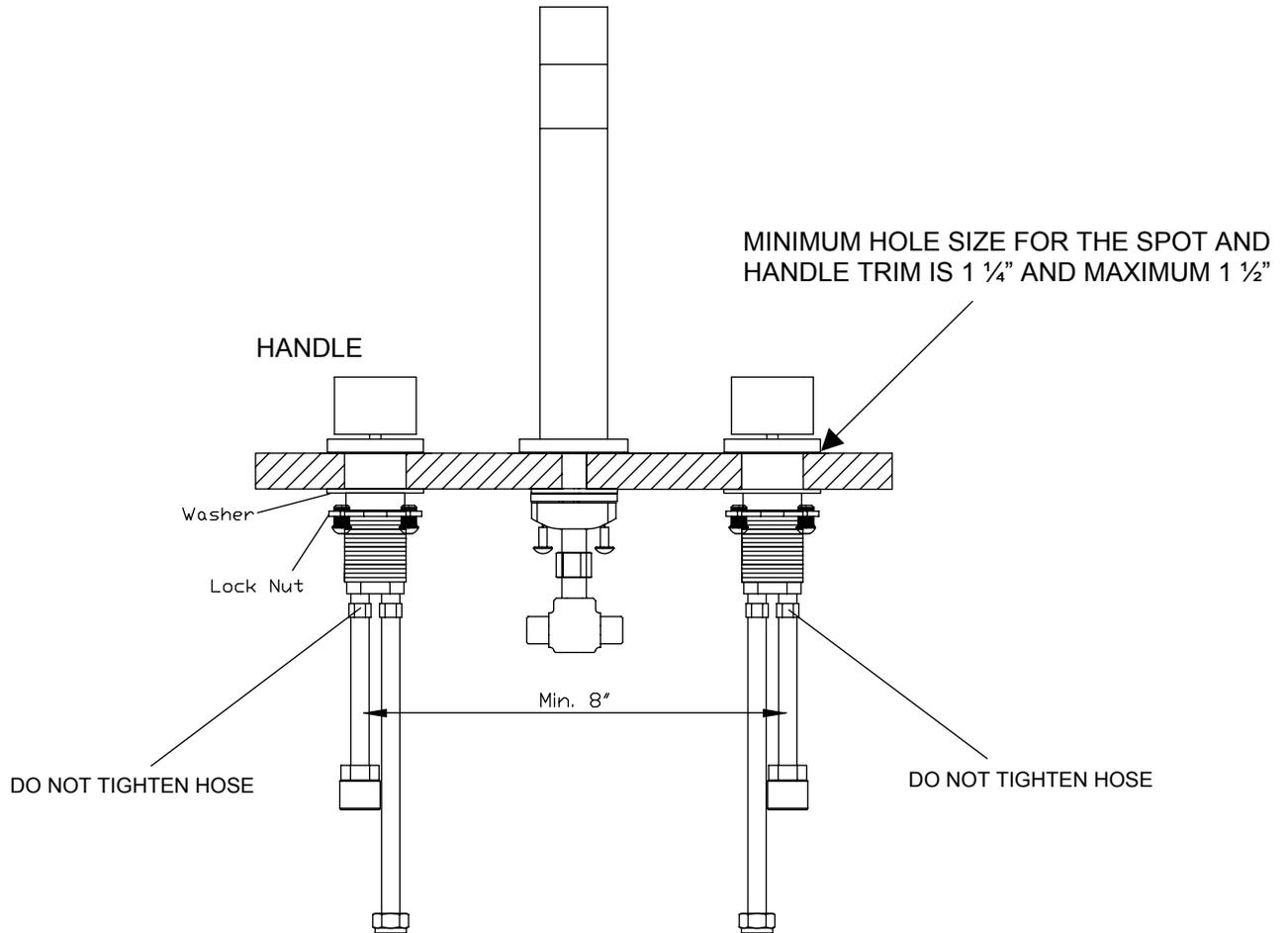
\*\*\* NOTE: SHUT OFF WATER SUPPLY BEFORE BEGINNING INSTALLATION\*\*\*
