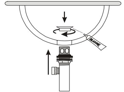
5. Insert drain plug into decorative drain flange with adjustable eye-screw facing back.
