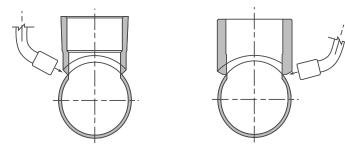
SPF Welded Outlets are designed to sit higher on the pipe, thereby requiring less weld and eliminating burn through. SPF Welded Outlets sit higher on the header or branch line pipe than competitive fittings. This allows the welding torch to remain in an optimum position for welding. In addition,  $1^{1}/2^{"}$  and larger female threaded and grooved welded outlets require the same hole size for installation. This results in fewer change overs when installed using automatic welders.
