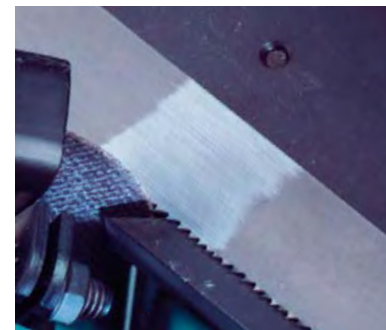
Removing excess weld from gullet (teeth) with cut-off wheel.
