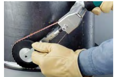
15420 tool (below) includes unique 11702 Contact Arm with hand guide.
