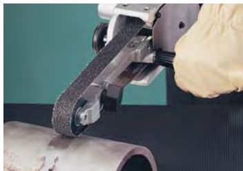
Model 11475 is ideal for grinding circumferential welds.
