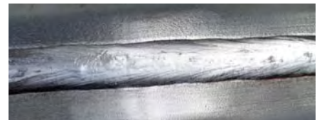
Weld seam cleaned with DynaRover.
