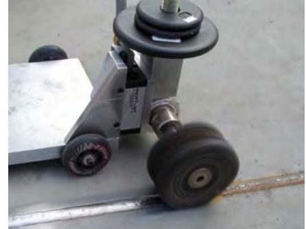
DynaRover cleaning a butt weld. (Shown with optional weight spindle.)
