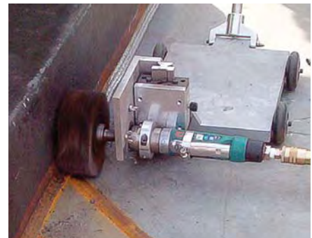
DynaRover cleaning an angle weld.
