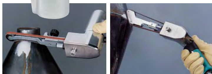
Slack of abrasive belt is used to efficiently polish radiused area.
