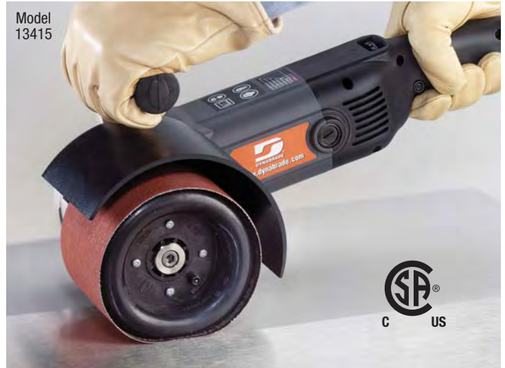
13415 Electric Dynisher® fitted with optional 92938 Dynacushion® Pneumatic Wheel and coated abrasive belt. An ideal setup for achieving in-line scratch pattern on stainless steel.
