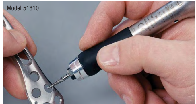
100,000 RPM Pencil Grinder offers enhanced cut rate.
