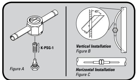
All Parker Sight Glass indicators are suitable for use with the halocarbon refrigerants, including 11, 12, 22, 113, 114, 134a, 404A, 407C, 410A, 502 and 507. Listed by Underwriter's Laboratories, Inc. for a working pressure of 650 psig or 4482 kPa.
