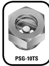
Types PSG-11S, PSG-13S, and PSG-17S have copper connections and feature a removable cartridge containing the moisture indicating element. The cartridge has a **knife edge joint** and is available as a separate unit for field replacement purposes if necessary. It is designed as PSG-10TS and fits all three sizes.
