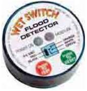
The Wet Switch is a solid state device designed to detect the presence of condensate water overflow. The Wet Switch is placed into the secondary drain pan — a normally dry pan. If the primary drain pan fails, condensate water will overflow into the secondary drain pan. Upon sensing moisture, the Wet Switch will turn the system off (typically the cause of the condensing water) to help prevent damage to carpets, walls, woodwork, ceilings, and other property.
