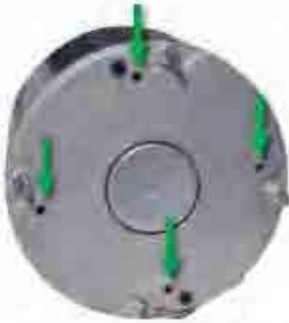
On RESCUE® 5.6" diameter motors lead end blind holes (4) are for mounting on Rheem® and Trane® units requiring grill mount motors. Special screws are provided.
