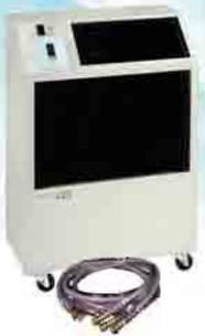
Provides 18,000 BTU of cool air. Space saving, quiet and powerful cooling. **A water cooled unit does not require condenser air ducting.** The rejected heat is transferred by the water leaving the water cooled condenser coil. 40' Hose kits are available for temporary installation or rental applications. Operates on standard 115v power.
