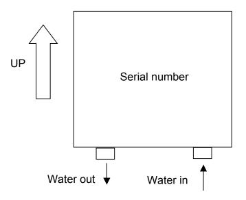
When correctly mounted, this "Series Two" water heating unit should look like the diagram to the left. <u>ANY</u> other mounting configuration will prevent the unit from operating properly.
