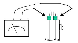
If the reading is less then 20 ohms on the single (Rx1) scale or the (Rx10) scale, then the element is good, if it is <u>much</u> greater.
