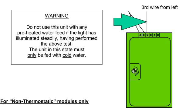
If the indicator light on the printed circuit board illuminates with the water flowing and there is no heating of the water, it is highly likely that the heating element has been damaged. If the above situation occurs, contact Technical Service for replacement elements.
