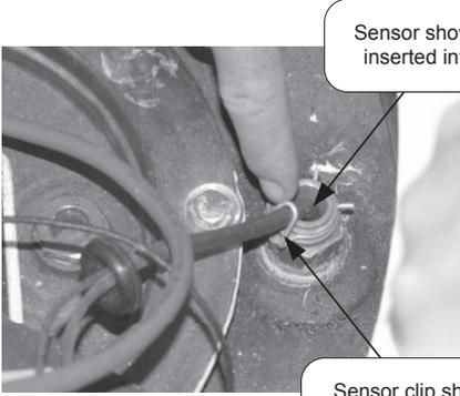
Sensor shown fully inserted into well
