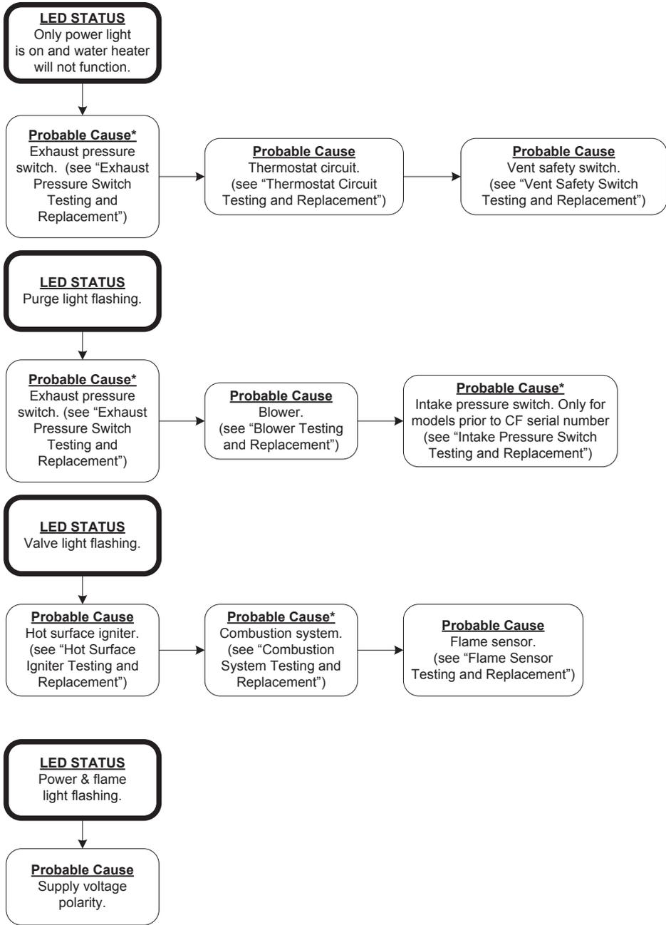
**Water Heater Fault:** Water heater does not operate
