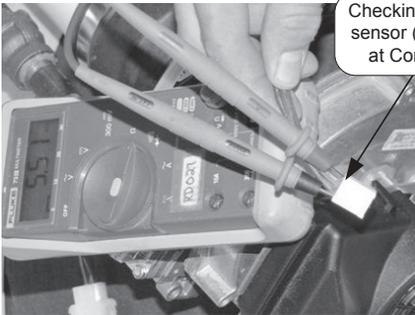
Checking continuity of sensor (disconnected at Control Board)
