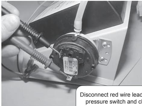
Disconnect red wire leads from pressure switch and check continuity through switch.
