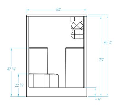
FEATURES Ibs Dimensional Tolerance ± 3/6". Dimensions needed for site preparation should be measured from the unit. Aquatic assumes no responsibility for preparatory work.
