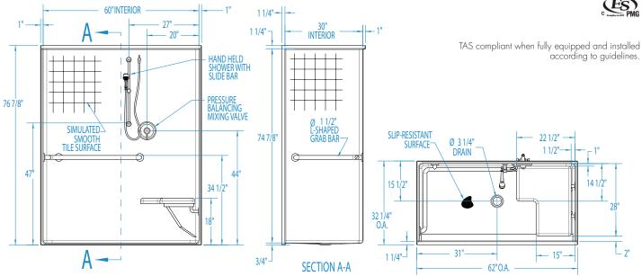
**FEATURES** Dimensional Tolerance ± %". Dimensions needed for site preparation should be measured from the unit. Aquatic assumes no responsibility for preparatory work.
