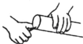
4. Remove dirt, grease and moisture; a thorough wipe with a clean dry cloth is usually sufficient. Moisture will retard cure and dirt or grease can prevent adhesion. Solvent cementing should not be attempted in the rain.
