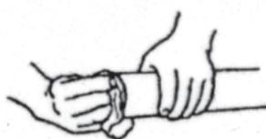
5. Check pipe and fittings for fit (dry) before cementing. For proper interference fit, the pipe must go easily into the fittings one-third to three-quarters of the way. Too tight a fit is not desirable. You must be able to fully bottom the
