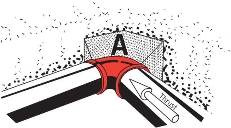
$$\text{area } A = \frac{\text{Thrust Force}}{\text{Bearing Strength of Soil}}$$
