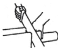
2. Plastic tube cutters may also be used for cutting plastic pipe. However, some cutters produce a raised bead at the end of the pipe. This must be removed with a file or reamer, as it will wipe the cement away when pipe is inserted into the fitting.
