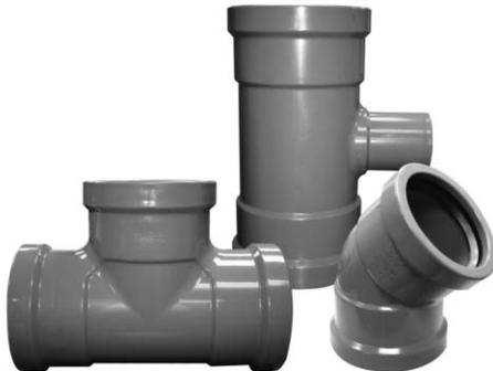
Blue Brute fittings are made to match PVC pipe, with the same deep bells and thick gaskets. In addition, Blue Brute fittings have removable gaskets so that oil resistant nitrile gaskets can be substituted when installing in contaminated soils.
