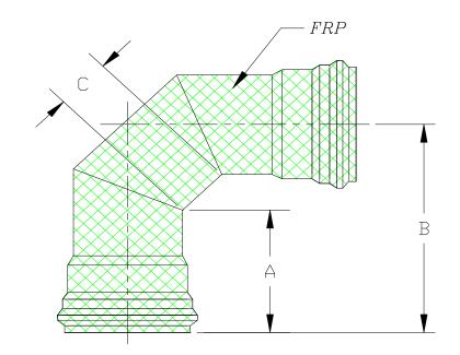
NOTE TO FABRICATORS: BE SURE TO WRITE ON THE ELBOW THAT THE "BELLS MUST BE GLASSED WITH 3M". THIS IS BECAUSE THE ELBOWS ARE MADE USING SDR26 MATERIAL INSTEAD OF SDR21.
