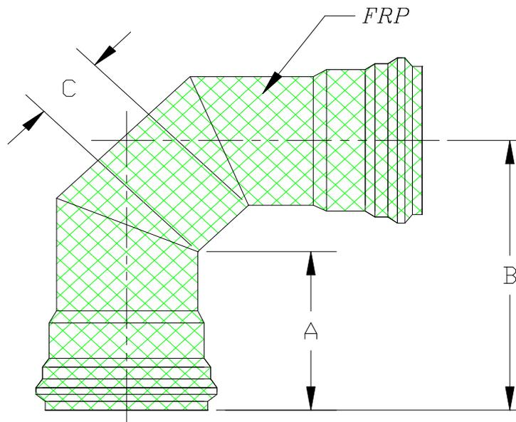
NOTE TO FABRICATORS: BE SURE TO WRITE ON THE ELBOW THAT THE "BELLS MUST BE GLASSED WITH 3M". THIS IS BECAUSE THE ELBOWS ARE MADE USING SDR26 MATERIAL INSTEAD OF SDR21.
