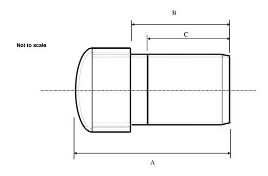
"B" Dimension is Critical...Measure the cap socket length and add B length to confirm cut length.
