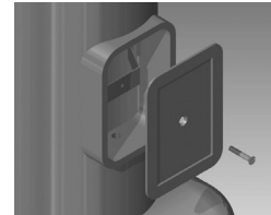
Handhole Detail Standard handhole assembly 4" x 6 -1/2"
