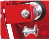
**Rope Deflector Sheave:** In the event that the rope should break the tension in the rope could cause severe injury – with the deflector sheave, the operator may stand well clear of the pulling equipment and in particular, the line of pull.
