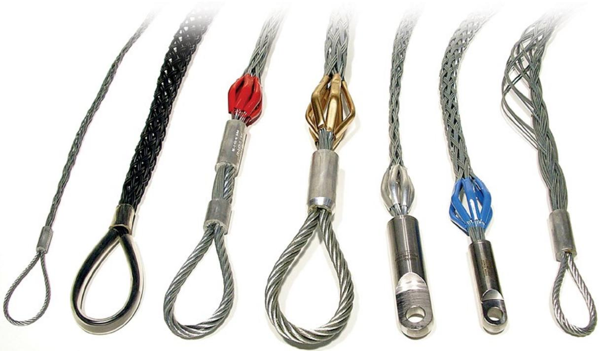
DCD cable grips are hand-woven by experienced trades-people guaranteeing a consistent level of high quality. DCD grips are reverse woven, creating a loop at the end of the grip instead of being soldered or crimped together (see photo inset below of typical grip end).
