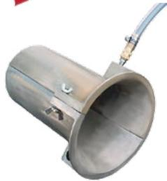
**Duct Entry Guide** (32500 series): This product fits right into the duct opening and has a roller that the cable must pass over. The unit is fitted with a spray nozzle that when hooked up, places the lubricant right onto the cable as it passes under the nozzle.
