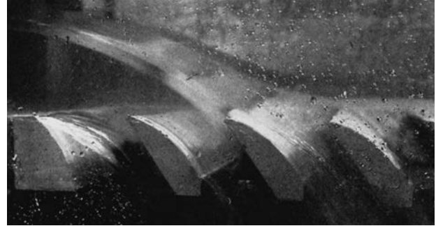
Cross section of Vane Style Grate in testing flume showing hydraulic performance at 2 cfs.
