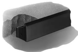
Cutaway from street, showing curb guard.
