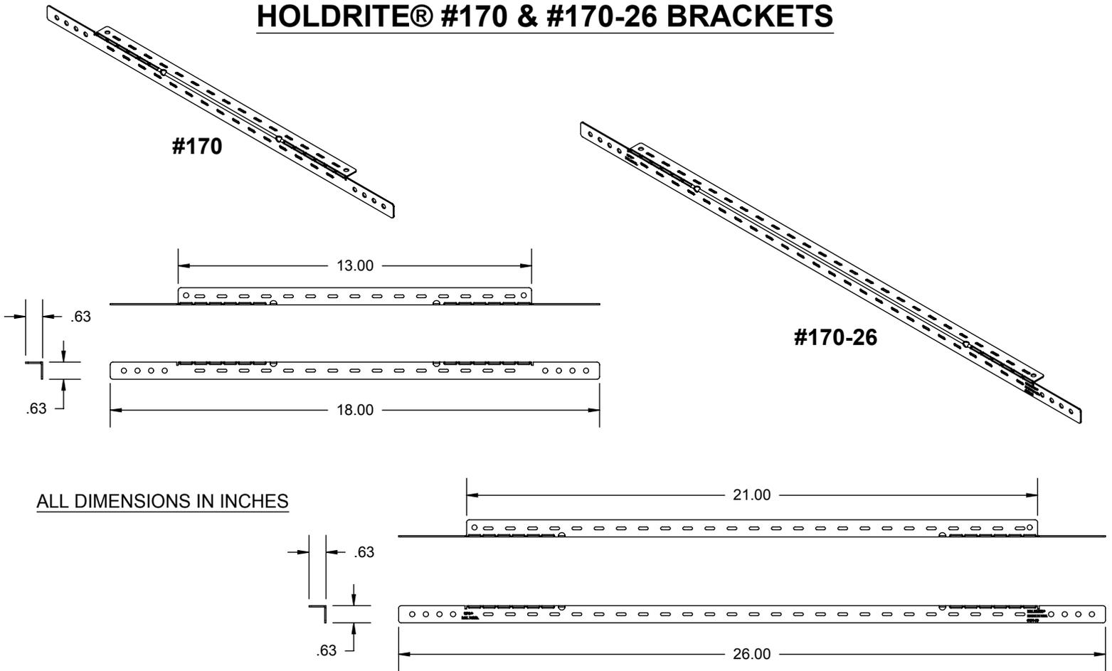
**Versatile, galvanized steel brackets providing a platform for horizontal or vertical tube support. Also ideal for shower head, diverter, tub spout and sink applications. Use HOLDRITE #251 Rapid Clamp™, Pro Clamp™, Stout Clamp™ and other industry clamps. Perforated tear feature allows brackets to fit into narrow stud bays. Bendable end tabs allow brackets to be recessed into stud or joist bays.**
