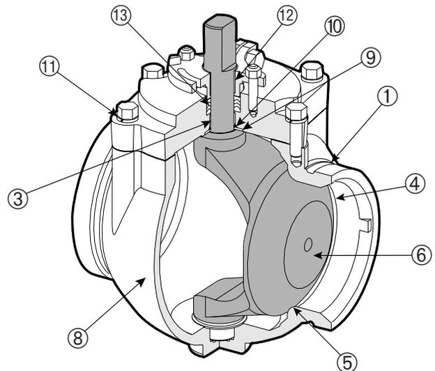
13. **Multiple Chevron Packing:** Provides a reliable, durable stem seal.
