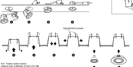
For dimming requirements, refer to dimmer manufacturer's specifications MR16 GZ5.3 bulb base configuration may vary between manufacturers resulting in various lengths of pins. DO NOT OVER PUSH AT INSTALLATION.
