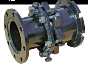
**NOTE:** Some initial axial movement may occur in lug style restraints as the lugs seat. Movement is directly related to the size of the piping system and the system pressure. In general terms movement of approximately 0.25 can be expected in restraints under 16". For larger sizes, movement of approximately 0.40 may be seen. If this is critical to your application please contact Romac Engineering for additional information.
