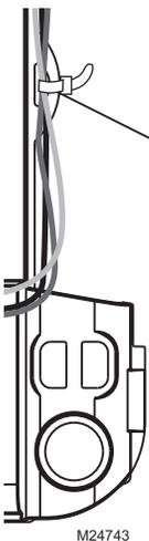
The HZ432 offers many innovations for wire management and organization: wires can be run behind the panel, through wire channels on its sides, and must be attached to a wiring anchor with a cable tie.
