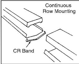
**SY920 Low Profile Wraparound** utilizes a shallow 3 1/4" housing. Self-spacing unit is suitable for low-density cellulose fiberboard ceilings.
