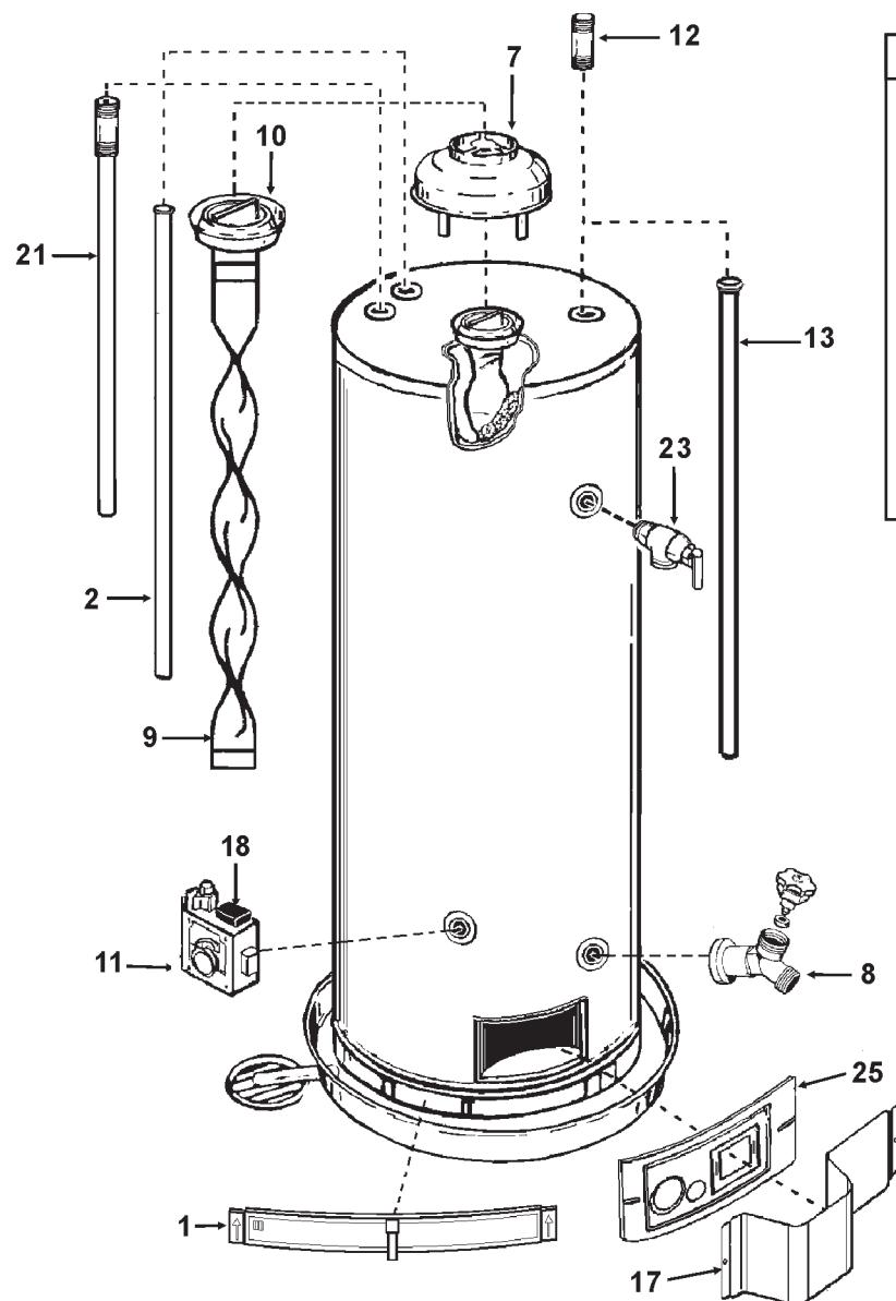
**BURNER ASSEMBLY****THERMOSTAT SHIELD****DRAIN PAN**
