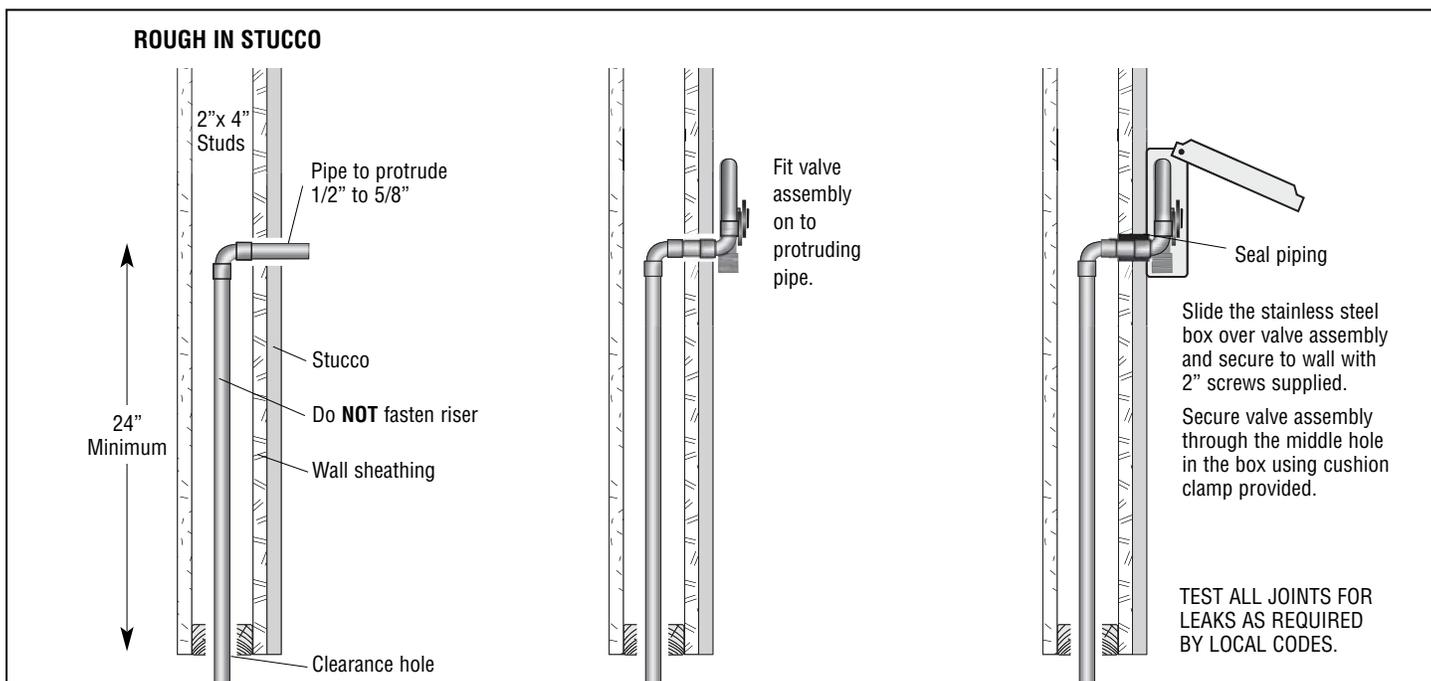
been installed on the piping system, slide the box over the assembly and fasten with screws provided.
