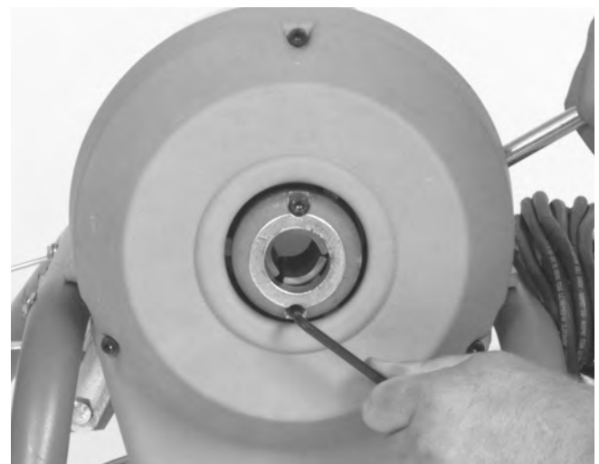
Figure 12 – Replacing Clutch Jaws
