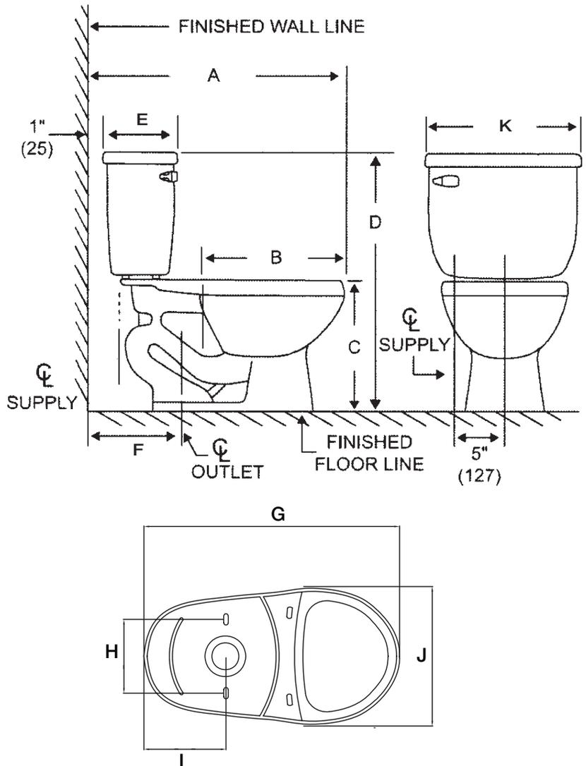
Note: All dimensions and specifications are nominal and may vary: Dimensions of 8" and greater have a tolerances of +3%. Dimensions less than 8" have a tolerances of +5%.
