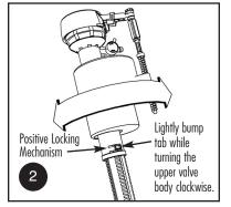
Familiarize yourself with the Positive Locking Mechanism and note how it locks the valve into position. No need to adjust now. HydroClean adiusts after installation
