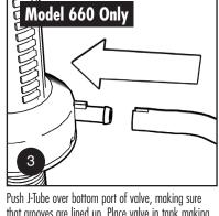
that grooves are lined up. Place valve in tank making sure the J-Tube lays flat on the bottom and up against the back and right hand side wall.
