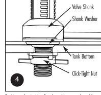
Position valve inside of tank making sure the rubber shank washer is seated as shown.
