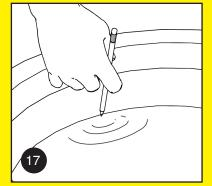
Use a pencil to mark 1/8" below water level in the bowl, then flush the toilet. If the valve is still filling the bowl after the water reaches the pencil mark, you will need to adjust the Mini-Valve to control the amount of water filling the bowl.
