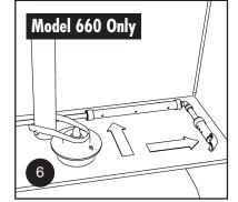
Make sure the J-Tube lays flat on the bottom of the tank, and is pushed up against the back and the right hand side of the tank.
