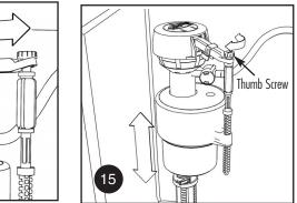
If you have turned off the water at the toilet, to fill the tank. Use the thumbscrew to adjust the proper water level inside the tank as indicated on the tank or 1/2" to 1" below the overfill tube.
