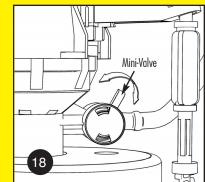
lydroClean ships with the Mini-Valve in the horizonta full open position. Turn counterclockwise to decrease the amount of water filling the bowl. Start with the valve in the middle position and adjust up or down until the tank shuts off close to the same time as the bowl hits the pencil mark.
