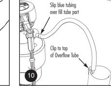
Install the single blue tubing with the clip, and attach clip to the overflow tube. Trim the blue tubing
