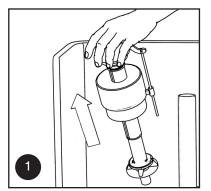
Shut water off, flush toilet to empty tank, and remove old toilet fill valve.
