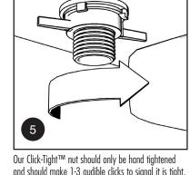
and should make 1-3 audible clicks to signal it is tight. The wings are engineered to bend if the nut is overtightened, preventing leaks and cracking.
