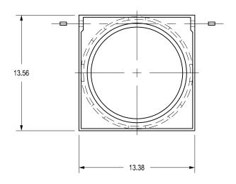
DIMENSIONS ARE FOR REFERENCE ONLY **ACTUAL DIMENSIONS MAY VARY** DIMENSIONS ARE IN INCHES GRATE MEETS H-20 LOAD RATING QUALITY: MATERIALS SHALL CONFORM TO ASTM A536 GRADE 70-50-05
