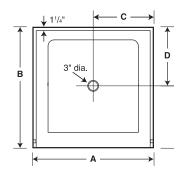
IMPORTANT: Rough-in dimensions are provided for reference only. You must measure the actual shower floor and check local building code requirements before construction of the stud wall.
