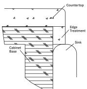
**Note:** Please consider and make allowance for the thickness of any edge treatment that surrounds the sink opening when determining Dimension "A".
