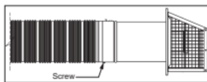
Figure 8 - Completed Vent Connection
