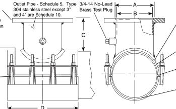
Outlet Gasket - Virgin Buna-N compounded for water service, per ASTM D2000. Outlet gasket assures complete seal of outlet area.
