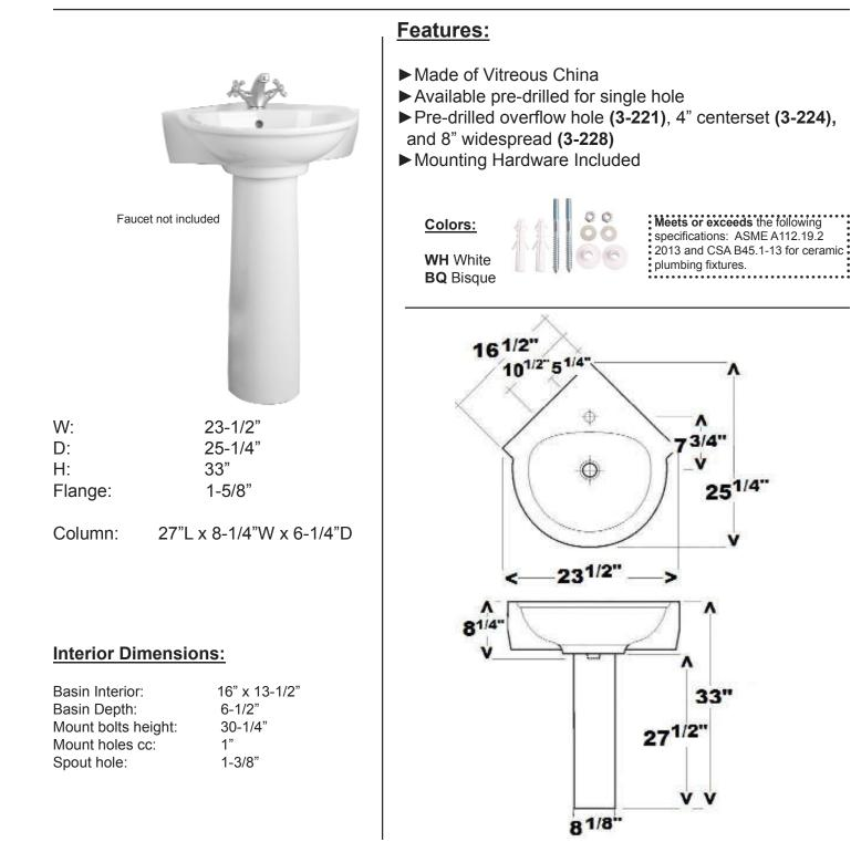
Dimensions of fixture are nominal and may vary within the range of tolerances established by ASMEI Standard A112.19.2-2013. Dimensions and specifications subject to change without notice.
