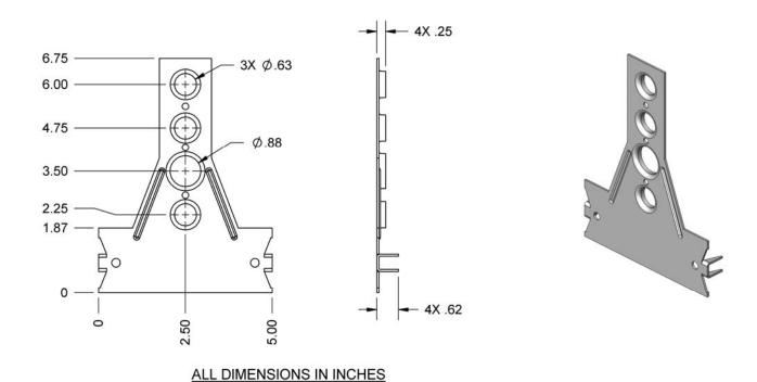
The HOLDRITE® #109-N-6 is a Copper-Bonded™ steel bracket made to position ½" or ¾" copper tube. Specifically designed to mount ½" stub-outs exactly 6" from the floor, with additional 5/8" holes at 2-1/4" and 4-3/4". There is a single 7/8" hole at the height of 3-1/2" for a hose bib, etc. This bracket also functions as a nail plate.
