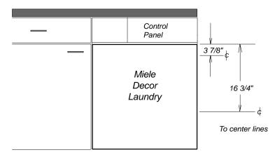
**Note:** To insure access to customer servicable features, a minimum 4" toe kick above finished floor (AFF) is required.
