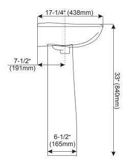
Note: All dimensions and specifications are nominal and may vary: Dimensions of 8" and greater have a tolerance of +3%. Dimensions less than 8" have a tolerance of +5%. Please utilize the current cutout template for countertop cutouts.
