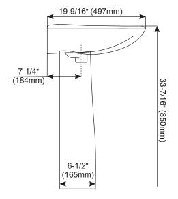
Note: All dimensions and specifications are nominal and may vary: Dimensions of 8" and greater have a tolerance of +3%. Dimensions less than 8" have a tolerance of +5%. Please utilize the current cutout template for countertop cutouts.
