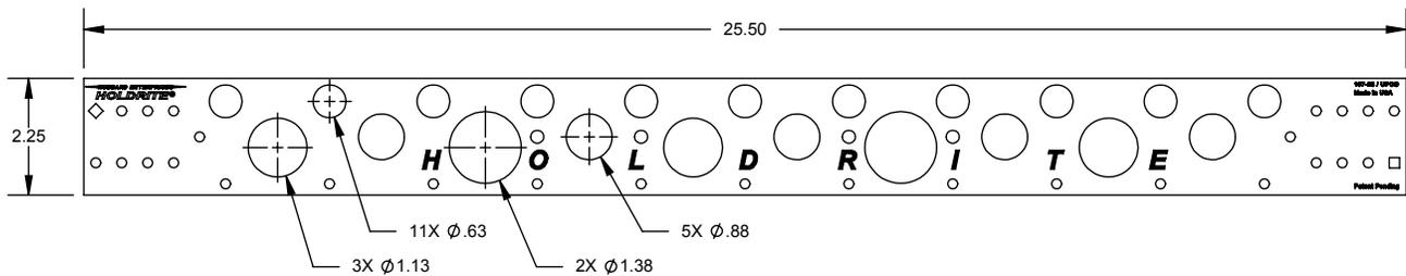
The HOLDRITE #107-26 is a Copper-Bonded™ steel bracket with holes for 1/2" tubings on 2" centers, holes for 3/4" tubings on 4" centers, holes for 1" tubings on 8" centers, and holes for 1-1/4" tubings on 8" centers.
