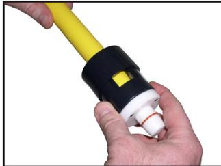
**4b** Chamfer end of pipe using [Continental's double ended ID chamfering tool](#).
