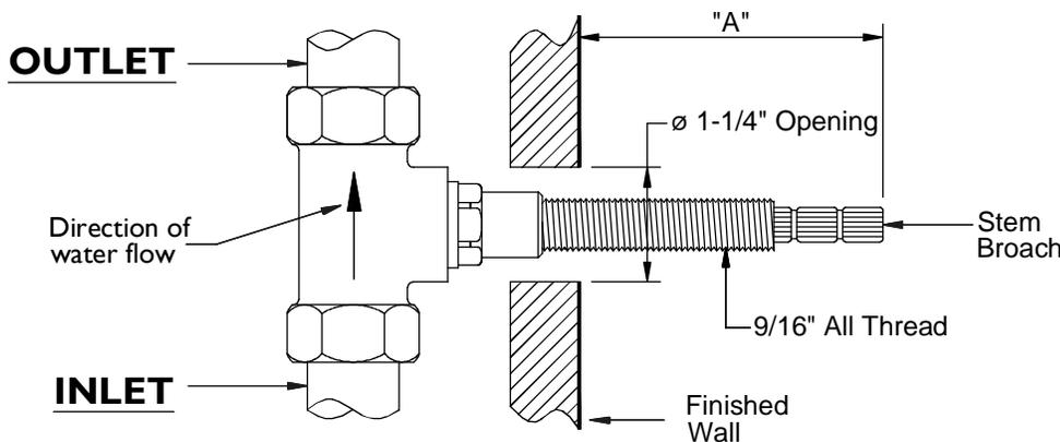
**NOTE: Valve must be installed according to direction of flow**
